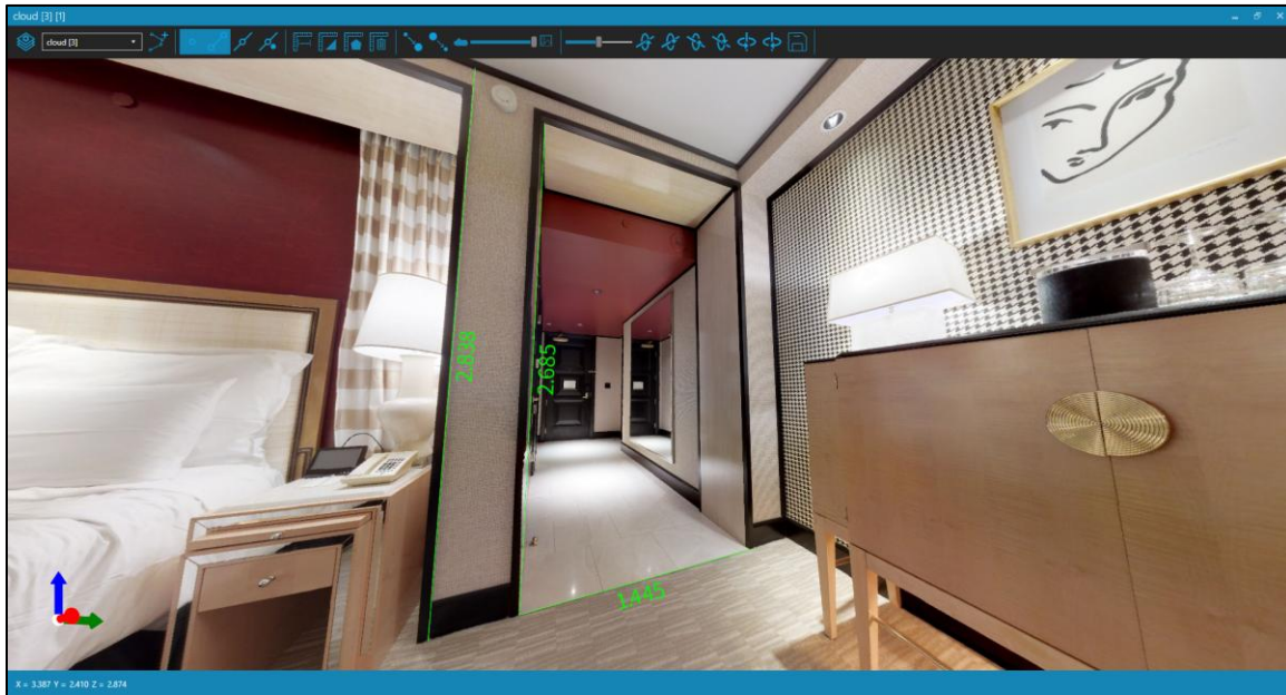
Figure 4. Precise measurement over image and point cloud in the background with Tcp PointCloud Editor
