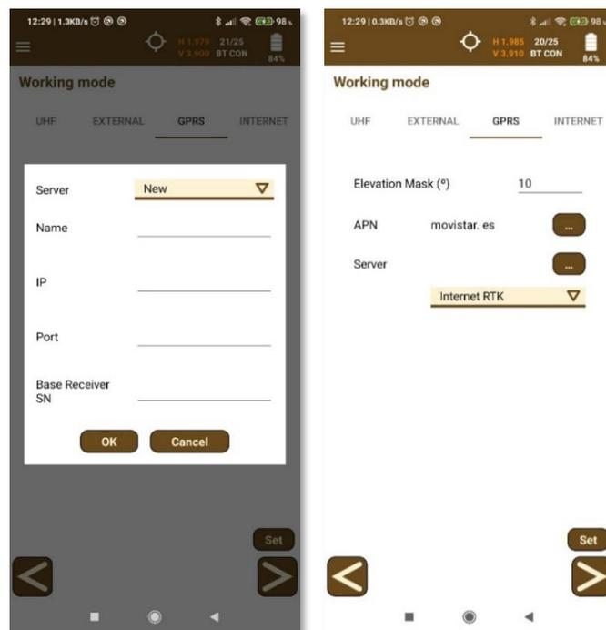
If the selected mode is NTRIP, the app asks for the caster parameters, such as **IP**, **Port**, **User Name**, **Password** and **Mountpoint**.
