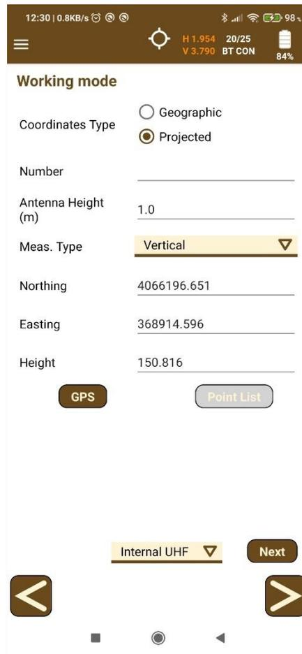
The **Number** or point ID, the **Antenna Height** and the base coordinates must be entered in the first configuration screen.
