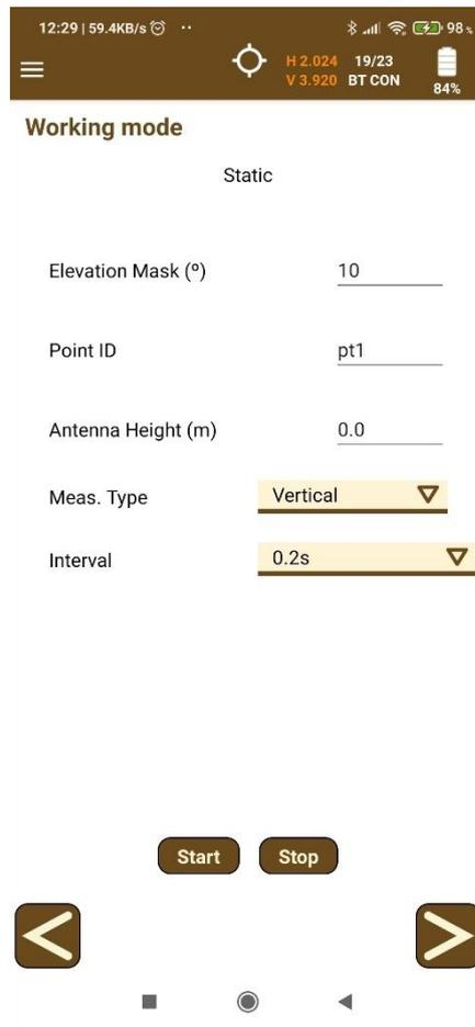
The **Point ID**, the **Elevation Mask** and the **Antenna Height** must be entered.
