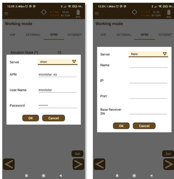
For APN, the app asks for the domain name, **User Name** and **Password** and, for iRTK server, it asks for **Name**, **IP**, **Port** and **Base Receiver** serial number.
