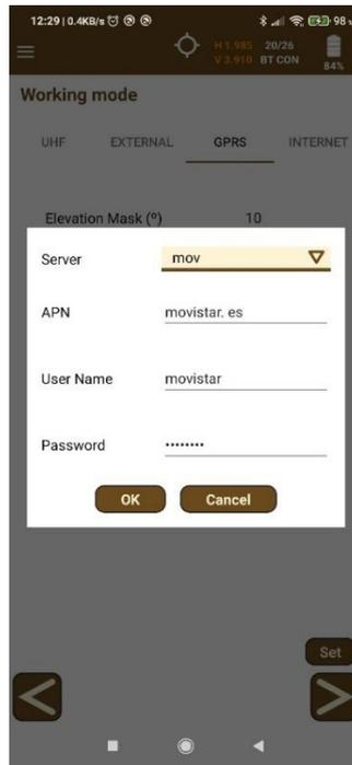
When selecting **iRTK**, the connection between base and rover is done connecting to a server through Internet. In this case, iRTK server parameter must be configured.
