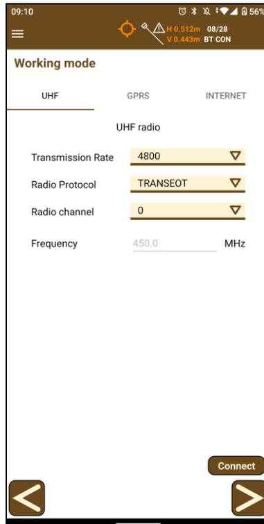
Figure 4. Rover UHF working mode
