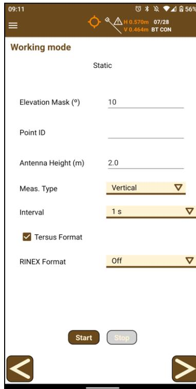
Figure 7. Static recording configuration
