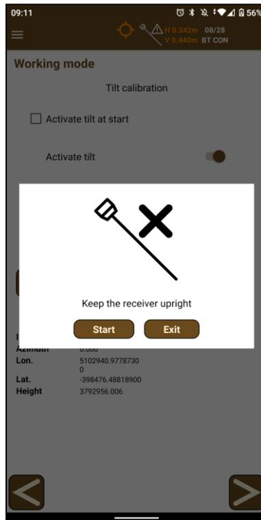
Figure 9. Tilt calibration dialog
