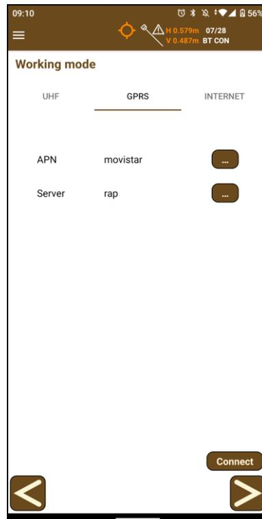
Figure 5. Rover GPRS working mode
