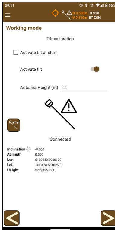
**Figure 8. Tilt start/stop screen**
