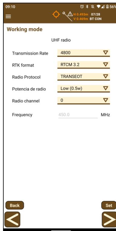
Figure 3. UHF Base working mode
