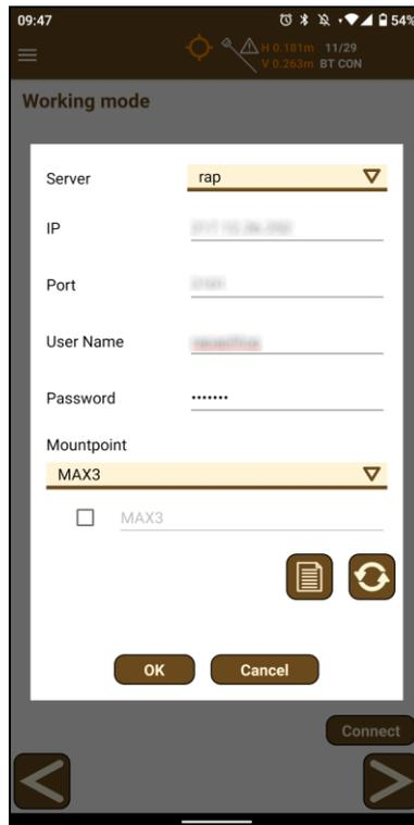
**Figure 11. NTRIP configuration**
