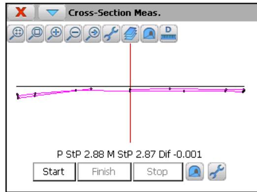
The station measured and the difference compared to the tunnel template are shown for each point read.
