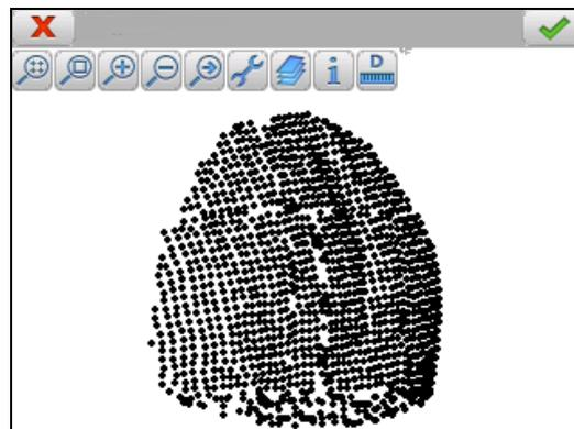
The program allows to measure and save points of the tunnel cross-section. Then, the program can **check control points**, orienting the total station automatically, getting the analysis with respect to the reference system and reporting the deviation from the theoretical point.
