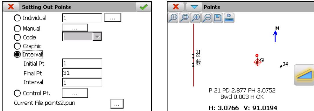
**Setting Out the Front.** The total station reads a point situated at the tunnel's excavation front, indicating the side and level desired. It analyzes the coordinates to subtract the station and searches the level's projection at the front through an iterative process until the 3D distance between the theoretical and measured points is less than the tolerance defined and provides information on the result obtained.
