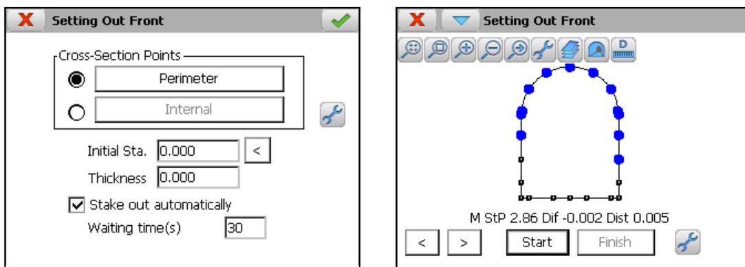
**Setting Out Cross-Sections.** Setting an interval and a tolerance of stations allows one to set out points of the tunnel's cross-section in each profile depending on the kind of increment indicated.
