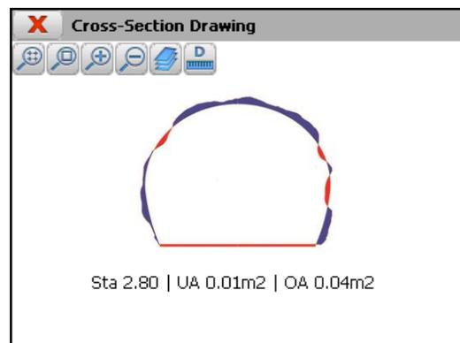
On screen are shown, in different colors, the under-excavation and over-excavation surfaces along with their numerical values calculated for each cross-section. Also, with motorized total stations, the program allows to rotate the instrument automatically to every point of the cross-section.
