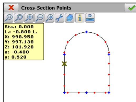
Tunnel templates can be simple or complex, and they can define by parameters, coordinates or points measured with total station. The tunnel template can be defined graphically by designating a polyline in **TcpTunnel CAD**.
