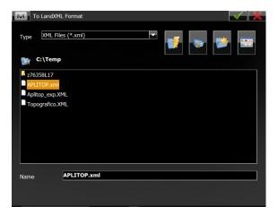
7. In following, specify the coordinate system to be used in the export, cross the box *Use Plane / Grid* and validate the dialog.
